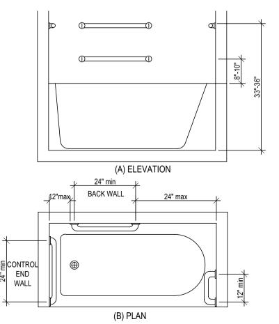
Aging-In Design note added For reinforcement installation: a) Reinforcement shall not be less than 2x8 nominal lumber or other construction material providing equal height and load capacity. Reinforcement shall be located between 32 inches and 39-1/4 inches above the finish floor flush with the wall b) Water closet reinforcement shall be installed on both side
