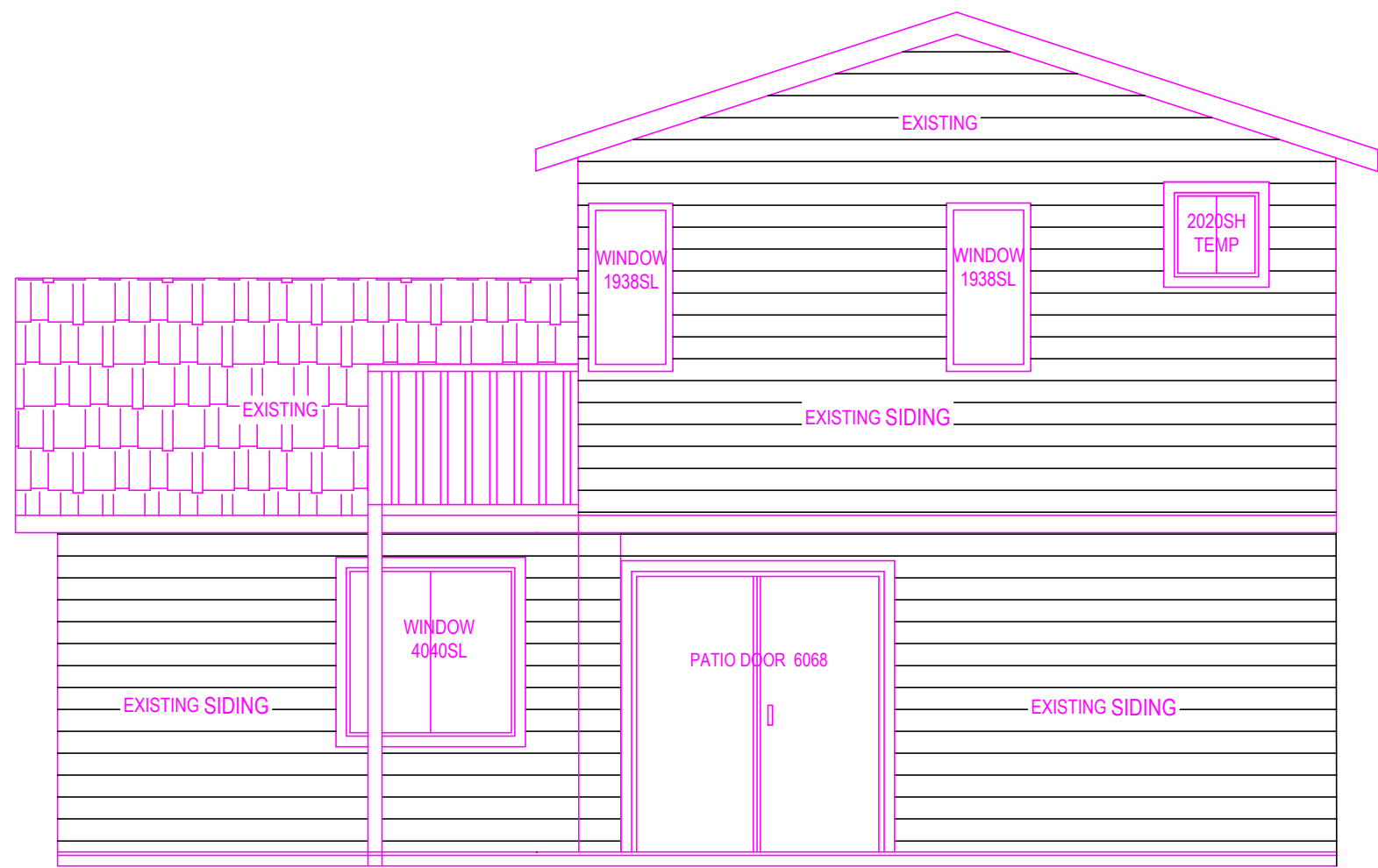
(E) REAR ELEVATION SCALE: 1 / 4" = 1'-0"
